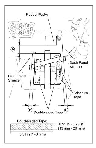
In the event the lower tibia pad has detached from the carpet, position the tibia pads on the floor panel and secure them using adhesive and double sided tape as shown.
